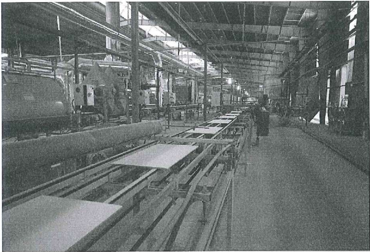
Conveyor system for transporting raw Tiles on the glazing and decorating line
