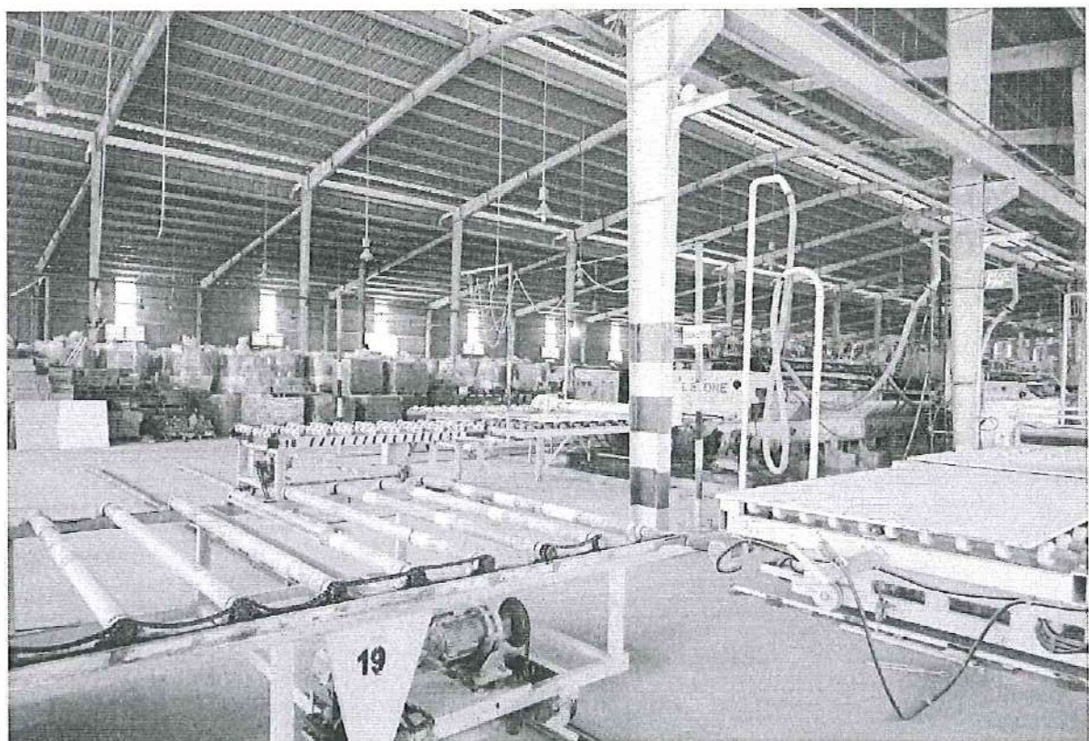
The conveyor system distributes the Tiles through the finishing and packaging line
