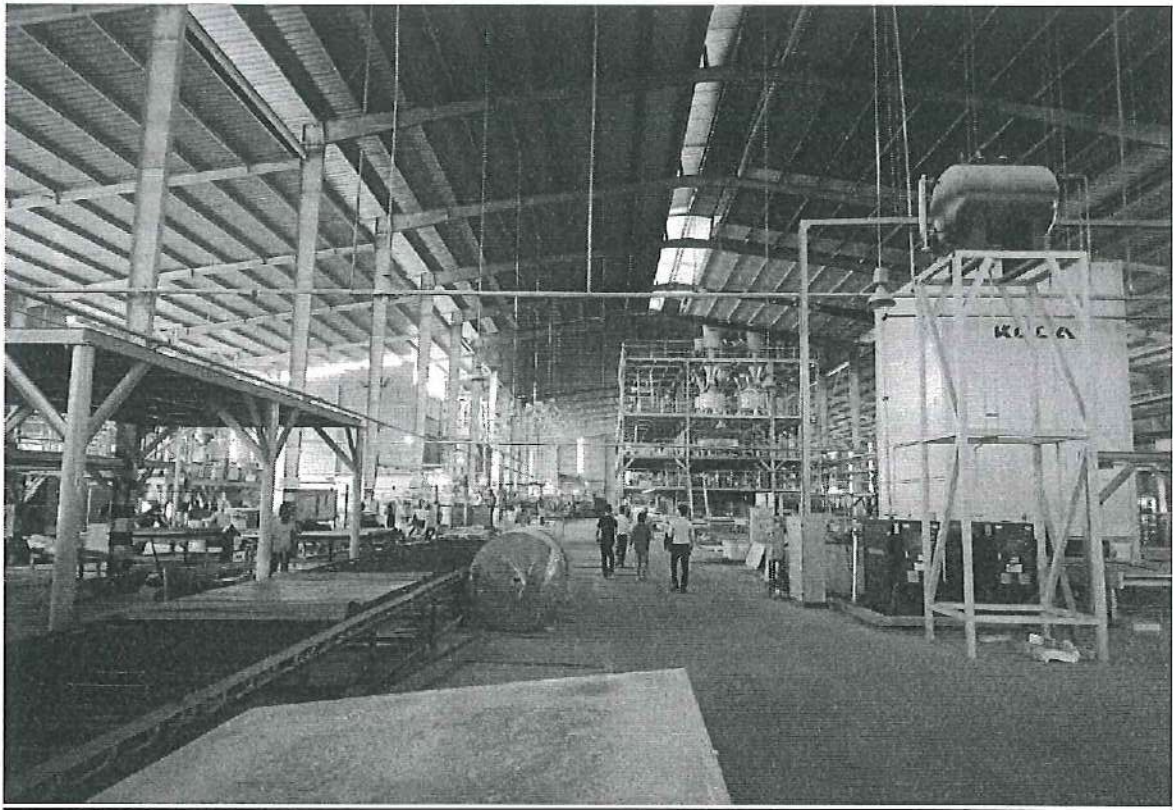
Spray drying tower system and powder preparation line for molding
